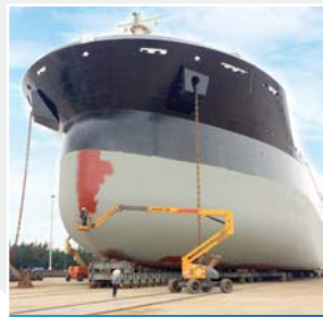
Painting & Blasting system • Painting hull ship • Abrasive steel blasting inside tanker
